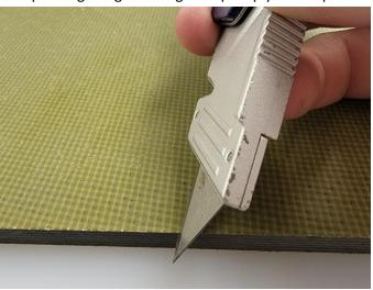
2.3 Using the dull side of the razor blade scrape near the cut and separate the peel ply from the carbon plate.
