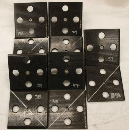
Fastener Pull-Thru Specimens post-test
