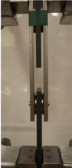
Beam Bearing Stress specimen in Test Fixture
