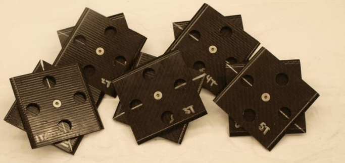
Fastener Pull-Thru Specimens pre test
