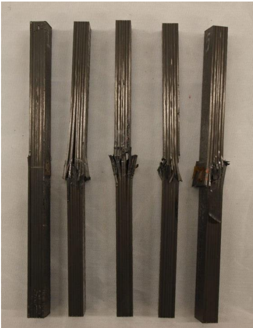
Beam Compression Post -Test
