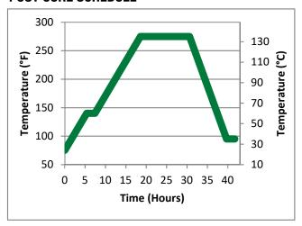
Post cure  $140^{\circ}F$  ( $60^{\circ}C$ ) x 2 hr +  $275^{\circ}F$  ( $135^{\circ}C$ ) x 12 hr with ramp rates no greater than  $12^{\circ}F/hr$ , to achieve maximum properties. For larger parts, additional dwells may be required.
