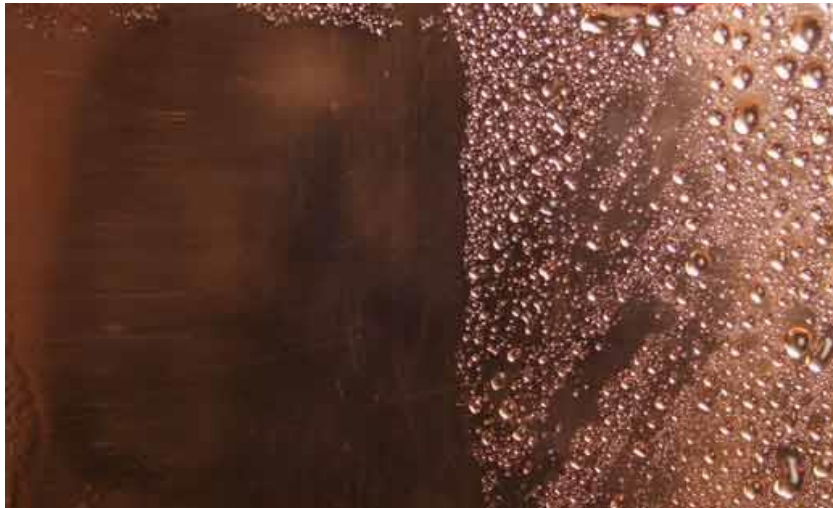
Left side is properly cleaned. Right side needs further cleaning.
