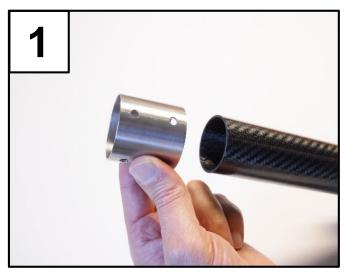
Slide the Drill Jig over the tube and tape in position
