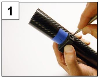
Align the bracket in the desired location and use a scribe to mark the mounting hole position
